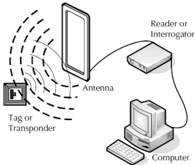
**Figure 1** How an RFID system works.
