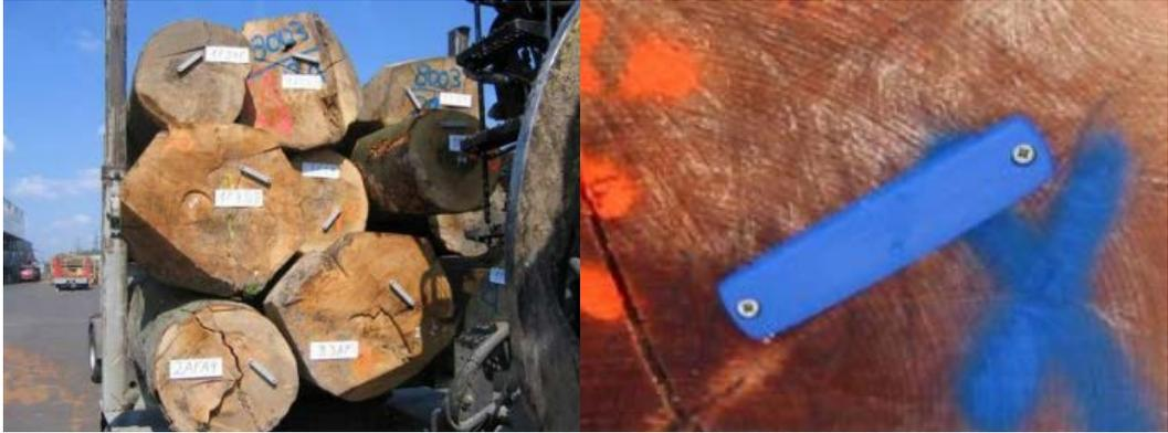
**Figure 2** Examples of RFID tags in forestry applications.
