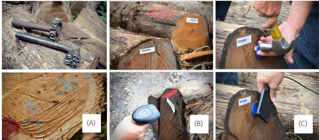
**Figure 3** Feasibility testing of RFID and barcoding in Thai forestry operations: (A) hammer branding; (B) barcoding; and (C) RFID.
