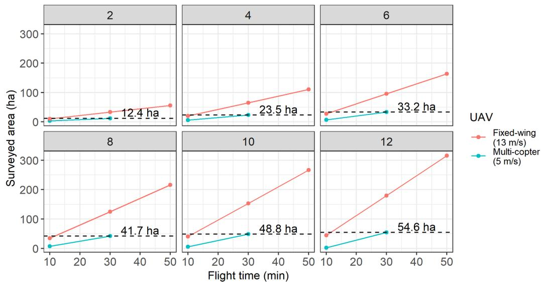
**Figure 3** Relationship between UAV flight time and maximum area coverage given the two different UAV platforms with GSDs of 2, 4, 8, 10, and 12 cm. Maximum area surveyed with a multicopter UAV is indicated by a dashed line for each GSD.
