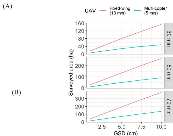
**Figure 4** Relationship between GSD and survey coverage of fixed-wing and multicopter UAVs at three different flight times (30, 50, and 70 min)
