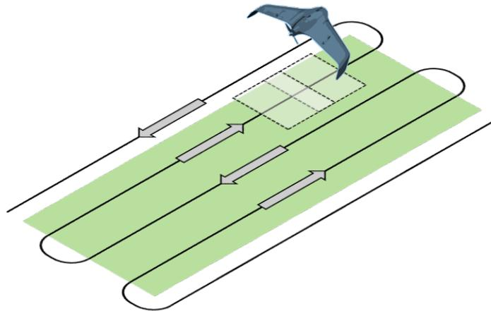
**Figure 1** Typical lawnmower pattern of the UAV-based mapping surveys. The area of interest is colored in green.
