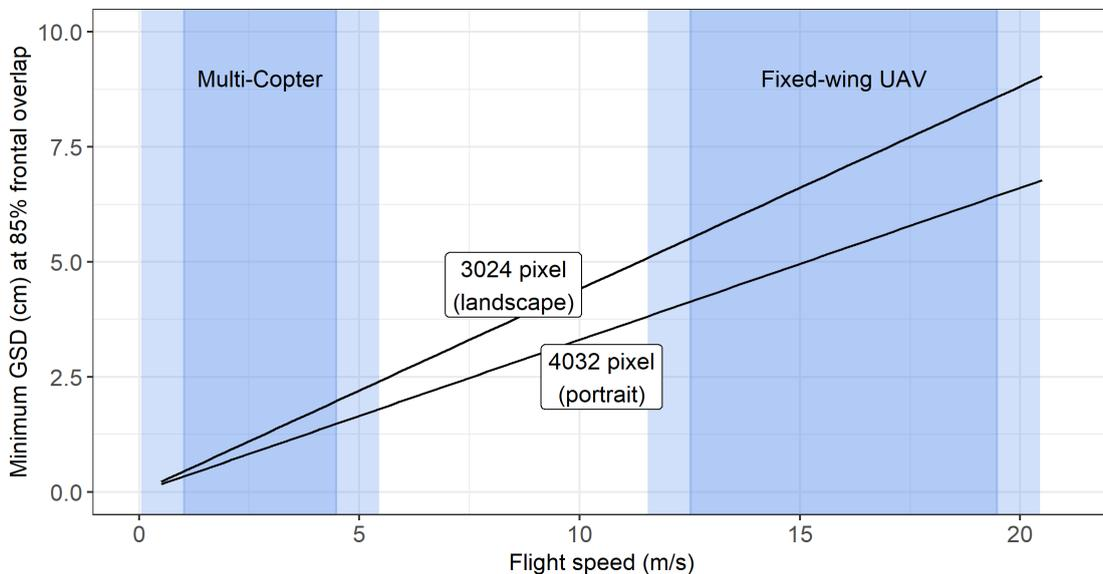
**Figure 2** Relationship between the flight speed relative to the ground and minimum possible GSD at which a frontal overlap of 85% can still be guaranteed using a commercial sensor with a size of  $3024 \times 4032$  pixels. Typical flight speed of multicopter and fixed-wing UAVs platforms are highlighted, respectively.
