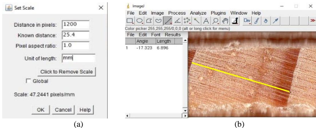
**Figure 1** Image scale setting (a) and ring width measurement (b) using the ImageJ software.
