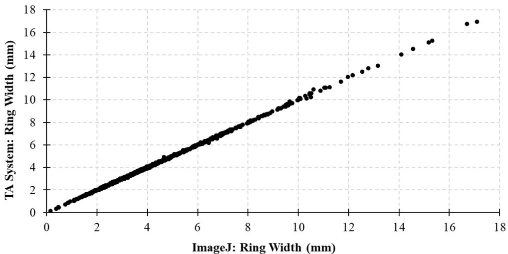
**Figure 4** Correlation between ring width data measured by TA System and ImageJ.
